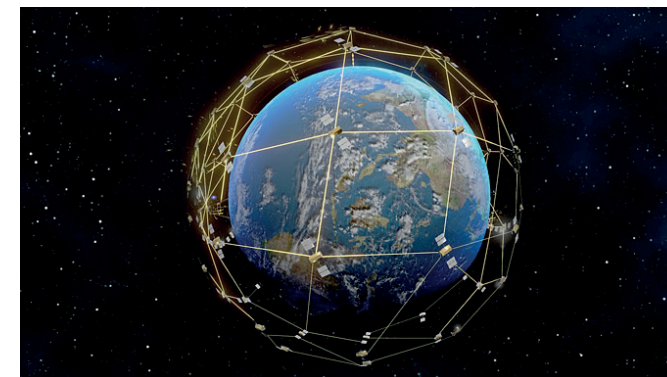
Figure 2: Example showing the global coverage of the Iridium satellite system. Iridium
